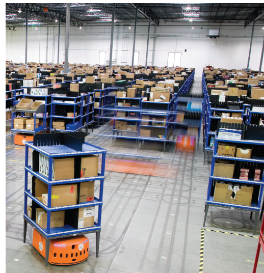
(b) A section of a KIVA equipped warehouse [4]
